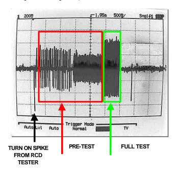
This 'spike' will, however, cause the 2100 to trigger and begin its reading cycle which will now be analysing the 'pre-test' section of the waveform. This will give incorrect measurements because of this.
